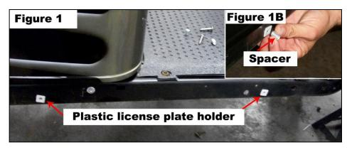
new rockers to the cart by screwing through the spacer and plastic license plate holder as shown in Figures 1B & 2.
